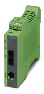
FO converter, for converting 10/100 BASE-T(X) to singlemode glass fiber, (1300 nm), SC duplex FO connection, rail-mountable, supply 24 V DC
